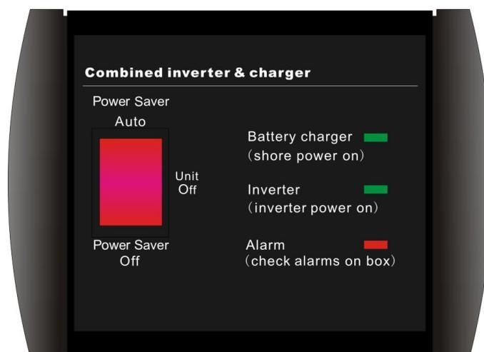
the inverter recognizes the need for power and automatically starts inverting and output goes to full voltage. When there is no load (or less than 25 watts) detected, the inverter automatically goes back into search mode to minimize energy consumption from the battery bank.
